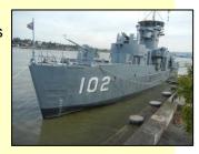
We saw how nearly 100 sailors were crammed into this 160-foot ship. These ships did not land material, but rather were specifically designed to give close-in fire support to marines landing on beaches. They had more firepower per foot (including four 40mm, four 20mm, and four 50 Cal guns, and 120 rockets) than any ships, and were nicknamed "mighty midgets".
